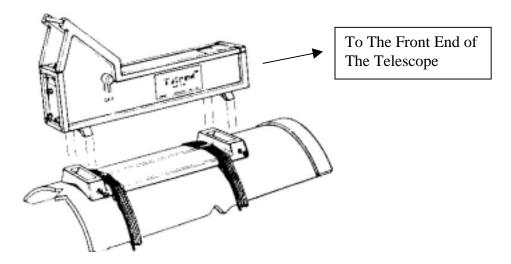
Placing the Telrad Unit In The Mounting Base
